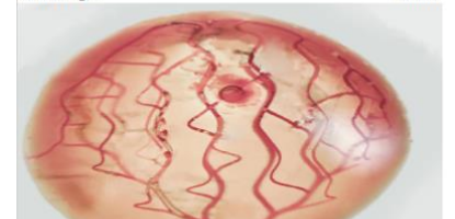
3D bioprinted soft tissue scaffold with vascularization channels perfused with red ink designed and produced using 3D Systems' and CollPlant's expertise and solutions.
