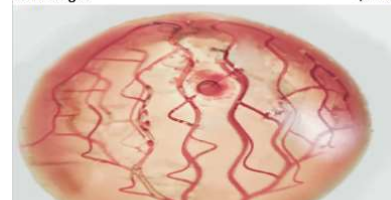
3D bioprinted soft tissue scaffold with vascularization channels perfused with red ink designed and produced using 3D Systems' and CollPlant's expertise and solutions.
