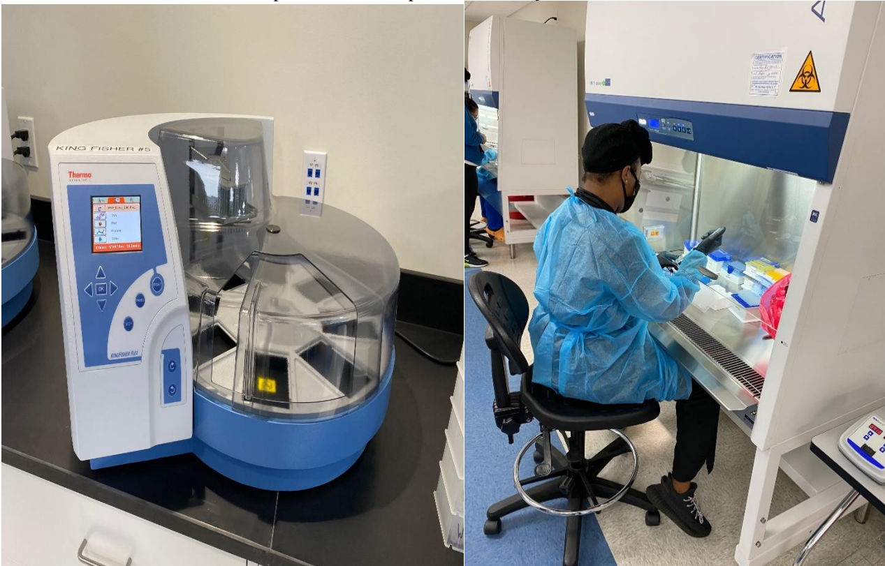
Exhibit 3. ThermoFisher Sample Prep System (left) and a Processing Station (right). These machines can process a 96 well plate in 22 minutes. Seven machines are operational with expansion underway to 18.
